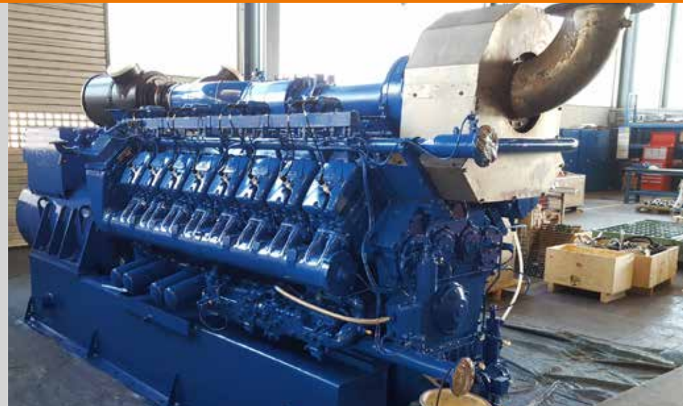
MWM gas engine after E70 general overhaul
